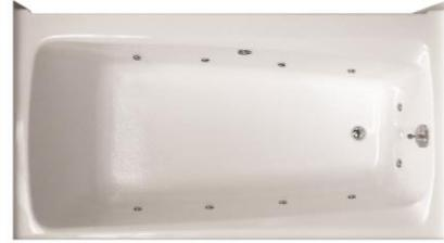
Warm Rain model WR 610AT (right hand plumbing) and WR 611AT (left hand plumbing) AirTubs are constructed of reinforced polyester resin covered with a high gloss gel-coat of 18 - 20 mil. thickness. The reinforced fiberglass has a minimum content of 18 % fiberglass.
