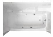
Warm Rain models WR 744SPD (right hand plumbing) and WR 745SPD (left hand plumbing) Front-Fit<sup>™</sup> remodeling tub/shower whirlpools are constructed of reinforced polyester resin covered with a high gloss gel-coat of 18 - 20 mil. thickness. The reinforced fiberglass has a minimum content of 18 % fiberglass. The bottom base of the unit is constructed of 1/2" end-grained balsa wood sandwiched between 2 layers of reinforced fiberglass. The base is an integral part of the unit.
