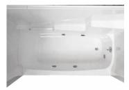
Warm Rain models WR 744ATD (right hand plumbing) and WR 745ATD (left hand plumbing) Front-Fit™ remodeling tub/shower AirTubs are constructed of reinforced polyester resin covered with a high gloss gelcoat of 18 - 20 mil. thickness. The reinforced fiberglass has a minimum content of 18 % fiberglass.
