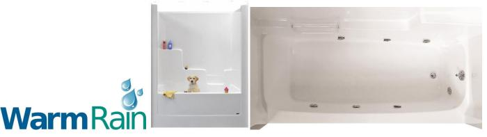
Warm Rain BIG OLE models WR 672SPD (right hand plbg.) and WR 673SPD (left hand plbg.) tub/shower whirlpools are constructed of reinforced polyester resin covered with a high gloss gel-coat of 18 - 20 mil. thickness. The reinforced fiberglass has a minimum content of 18 % fiberglass.
