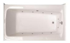
Warm Rain Melissa model WR 612AT (right hand plumbing) and WR 613AT (left hand plumbing) AirTubs are constructed of reinforced polyester resin covered with a high gloss gel-coat of 18 - 20 mil. thickness. The reinforced fiberglass has a minimum content of 18 % fiberglass.
