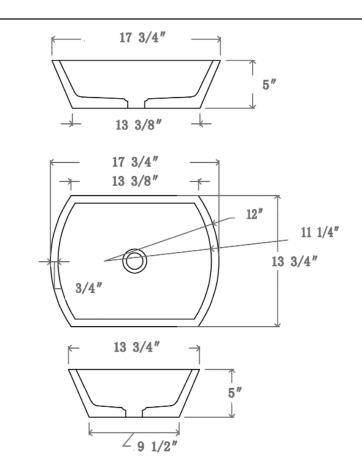
Dimensions of fixture are nominal and may vary within the range of tolerances established by ASME Standard A112.19.2. Dimensions and specifications subject to change without notice.
